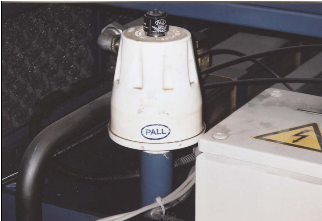
FIGURE 9. Good quality filters with absolute micron ratings, such as Pall or Harvard filters, are recommended for use in all hydraulic applications.
