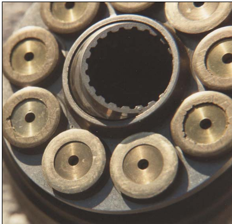
FIGURE 5. A piston pump assembly illustrating the severe scoring visible on the piston slipper faces. Note the mushroomed edges of some of the slipper faces. This is indicative of a lack of sufficient lubricant film between the slipper face and swash plate and suggests that the drilled lubricant passage in the piston was plugged with contaminants.
